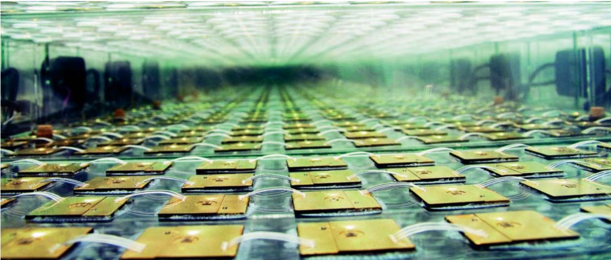
Sunlight is concentrated on the high efficiency III-V multiple solar cells
